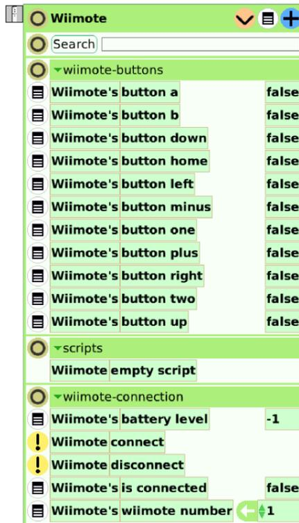
In a special category called “Wiimote-connection” we can find instructions which are useful for connecting with the Wiimote. In order to change categories we have to double click the tiny triangle which is on the left hand side of the title of the categories (for instance “Wiimote-buttons”) and then we have to choose the desired category.
